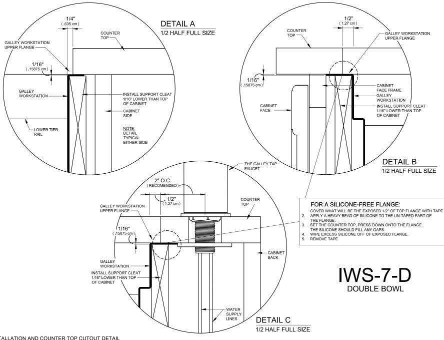
INSTALLATION AND COUNTER TOP CUTOUT DETAIL SHEET 2 OF 2
