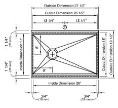
SUGGESTED GALLEY TAP PLACEMENT GUIDE Suggested maximum inside corner radius of countertop cutout 3/8" <sup>(6)</sup> Galley Tap 13/8" min to 1 1/2" max hole diameter Center Tap hole diameters 2" behind cutout Note: Salley Hot & Cold Tap requires a minimum 8" clearance to center if installed to the right of the Galley Tap Note: Tap Placements are for right hand or left hand drain orientation
