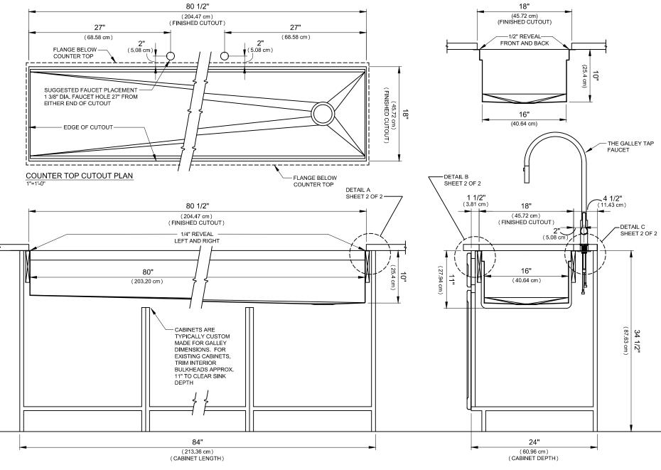
INSTALLATION AND COUNTER TOP CUTOUT DETAIL SHEET 1 OF 2
