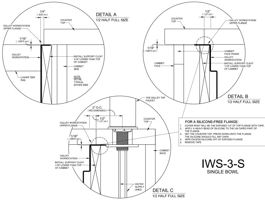
INSET CABINET INSTALLATION AND COUNTER TOP CUTOUT DETAIL SHEET 2 OF 2
