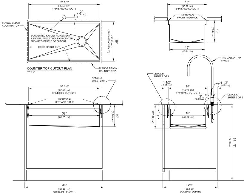
INSET CABINET INSTALLATION AND COUNTER TOP CUTOUT DETAIL SHEET 1 OF 2
